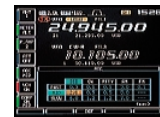
Example for setting the time constant for SSB-Mid, 2.0 seconds.
